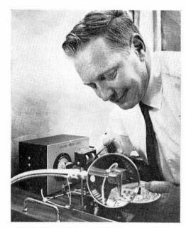
BERNARD STIEFELD (5425) demonstrates new technique to test electroplated holes in printed circuit boards. In magnified area, the "jaw" of the device is positioned over a hole. A 0.1 ampere constant current is applied and the output signal through the hole is a measure of the thickness of the electroplating.
